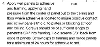
5. Finish head drywall screws may be used in the center of the panels to insure contact.
