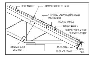
B. Starting at low or outside edge of the roof, place the panel on the bar joists with groove edge toward low portion of roof and tongue toward high portion. Fasten using Olympic #14-10 Heavy All Purpose screws (or equal) 1-1/2" from edges and one in the center (12" from edge at each bar joist location (3 screws per joist), see diagram on top of page 2. To install pre-drill hole through panel into flange of the steel joist using 7/32" high-speed
