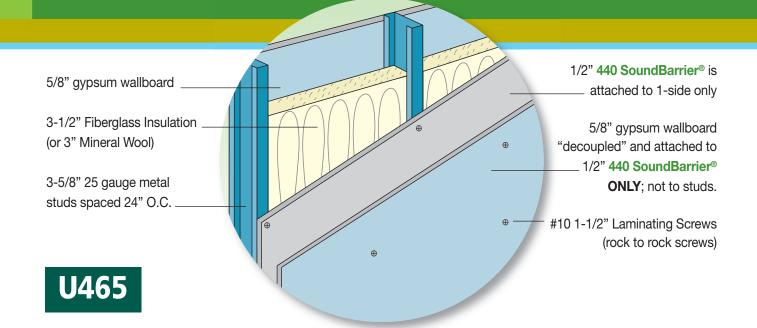
\* A similar wall with 2 layers of our competition's product<sup>†</sup> achieves an STC rating of 49, while a single layer of Homasote 440 SoundBarrier<sup>®</sup> achieves an STC rating of 55.
