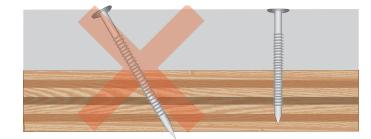
Drive 1" threaded nails or coarse threaded screws straight into subfloor, but not through the subfloor.
