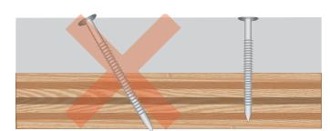
7 Drive 1" threaded nails or coarse threaded screws straight into subfloor, but not through the subfloor.
