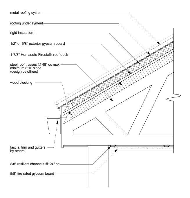
Firestall® Roof Deck Detail FS-MRD-ID-178-48-27 UL Design No. P535
