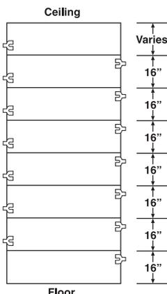
floor where adhesive is located to insure positive contact, and screw panels 6" o.c. to plates or blocking at floor and ceiling. Screws should be of sufficient length to penetrate 3/4" into framing. Hold screws 3/8" back from edge of panels. Screw clips to framing and brace panels for a minimum of 24 hours for adhesive to set.
